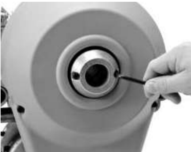
Figure 11 – Replacing Clutch Jaws
