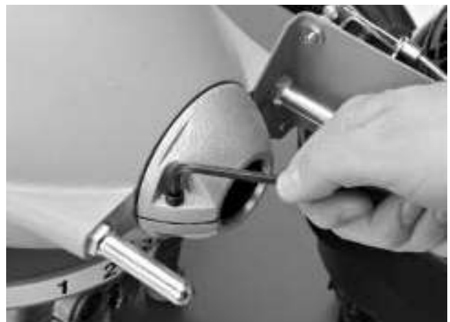
Figure 13 – Removing Clutch End Play
