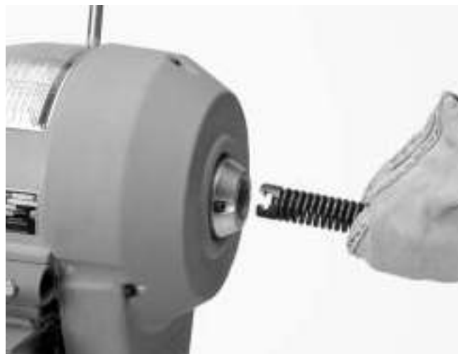
Figure 3 – Inserting Cable Into Front Of Machine
