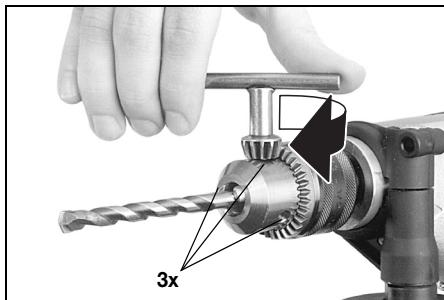
**Chuck the tool:** Insert the tool and use the chuck key to uniformly clamp tight all 3 bores.
