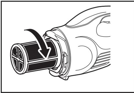
Connect capsule. Align O symbol on capsule with O symbol on handle and then firmly twist capsule in direction of arrow until it is secured.
