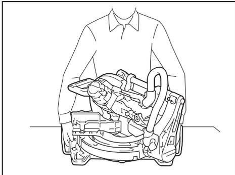
**⚠WARNING: Stopper pin for carriage elevation is for carrying and storage purposes only and not for any cutting operations.** The use of the stopper pin for cutting operations may cause unexpected movement of the saw blade resulting in kickback and serious personal injury.
