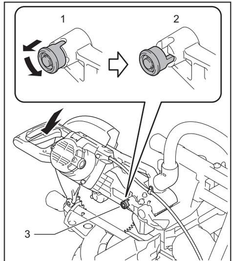
► 1. Locked position 2. Unlocked position 3. Stopper pin
