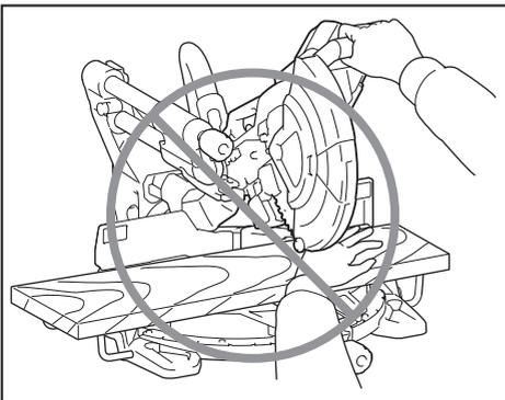
6. **Do not reach behind the fence with either hand closer than 100 mm from either side of the saw blade, to remove wood scraps, or for any other reason while the blade is spinning.** The proximity of the spinning saw blade to your hand may not be obvious and you may be seriously injured.
