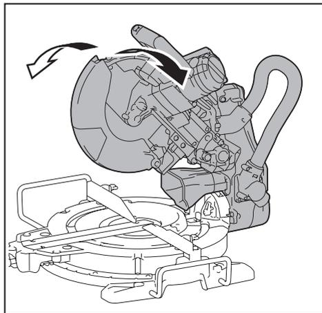
If the pointer does not indicate the 45° position, align it with 45° position by turning the adjusting bolt on the opposite side of the bevel angle scale.
