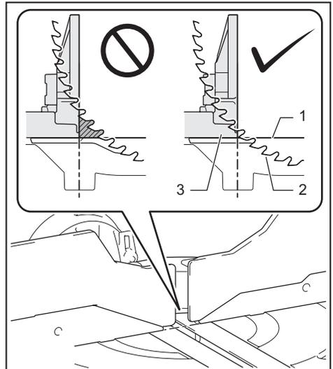
► 1. Top surface of turn base 2. Periphery of blade
