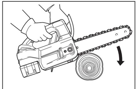
When cutting thick branches, first make a shallow undercut and then make the finish cut from the top.
