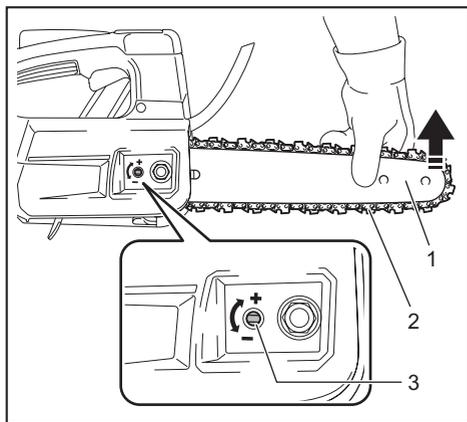
► 1. Guide bar 2. Saw chain 3. Chain adjusting screw
