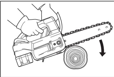
2. With the saw chain running, saw into the wood while using the top handle to raise the saw and the front one to guide it.
