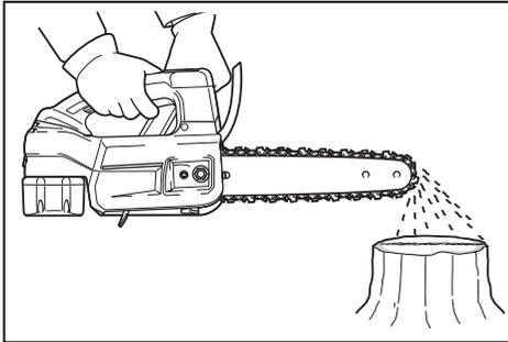
**NOTICE:** When filling the chain oil for the first time, or refilling the tank after it has been completely emptied, add oil up to the bottom edge of the filler neck. The oil delivery may otherwise be impaired.
