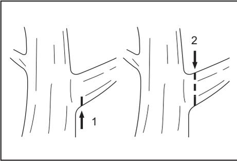
If you try to cut off thick branches from the bottom, the branch may close in and pinch the saw chain in the cut. If you try to cut off thick branches from the top without a shallow undercut, the branch may splinter.
