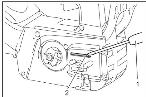
► 1. Slotted screwdriver 2. Oil discharge hole
