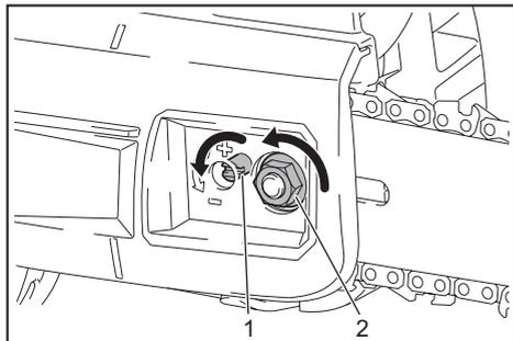
► 1. Chain adjusting screw 2. Retaining nut
