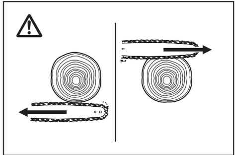
When you cut a wood under tension, cut the pressured side (A) first. Then make the final cut from the tensioned side (B). This prevents the bar from becoming trapped.
