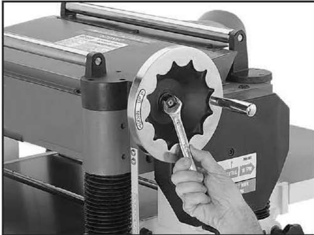
Figure 9. Installing the table height handwheel.
