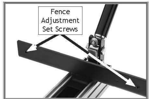
Figure 118. Location of set screws to adjust fence parallelism (shown upside down).
