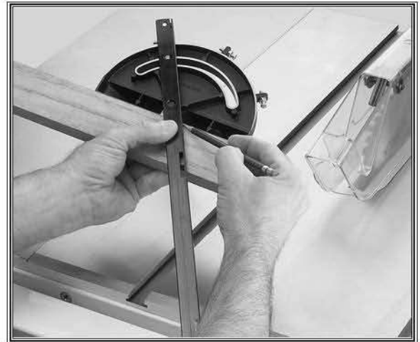
Figure 58. Example of marking miter line.
