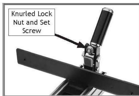
Figure 117. Set screw for adjusting fence handle clamping pressure.
