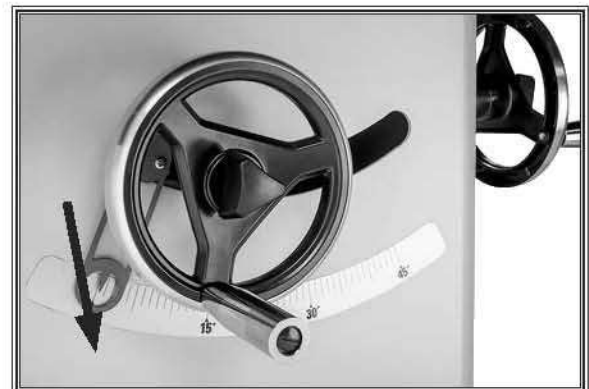
Figure 100. Tilt indicator arrow location.
