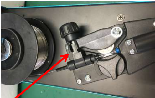
[7-9] Close down the top roller bracket and clip the pressure arm into place. Apply a medium amount of pressure to the drive roller
