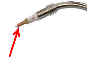
[13/14] Fit the correct size contact tip over the wire and fasten tightly into tip holder
