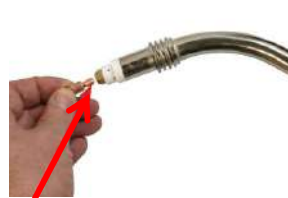
[10] Remove the gas nozzle and contact tip from the front end of the MIG torch
