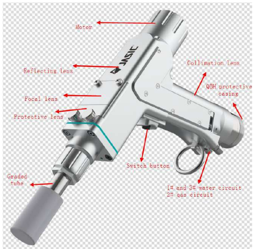
Figure 2-1 Handheld laser welding torch diagram
