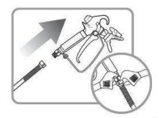
Attach Paint Hose to Paint Gun and tighten with two wrenches.
