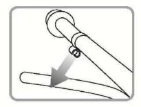
1. Separate smaller Priming Tube from Suction Tube.
