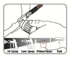
Start spraying at the lowest setting on the Pressure Control Knob and increase pressure as needed by turning clockwise to create a good spray pattern.
