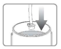
8. Remove Suction Tube from water or flushing solvent and submerge in paint pail.
