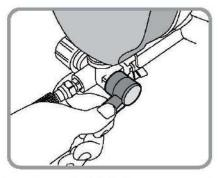
Turn Spray/Prime Switch to Spray mode and continue to spray into waste bucket.
