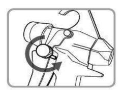
4. Turn Trigger Lock Knob to Locking position.
