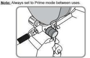
Point gun into paint pail and activate Sprayer Trigger to relieve pressure.
