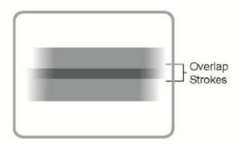
Overlap strokes by half, always aim stroke at bottom edge of last stroke.
