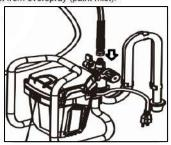
Attach Paint Hose to Paint Hose Outlet and tighten with wrench.
