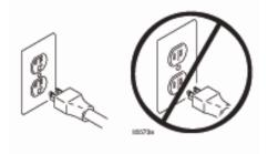
Do not use the sprayer if the electrical cord has a damaged ground contact. Only use an extension cord with an undamaged ground contact.
