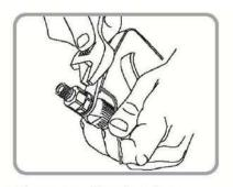
13. Remove trigger guard from housing.
