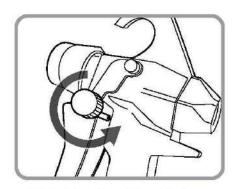
12. Stop spraying and activate trigger lock.
