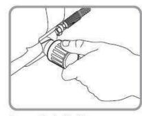
Turn Pressure Control Knob to Low Pressure Spray setting.
