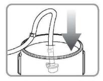
4. Submerge Suction Tube in water or flushing fluid.
