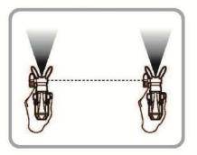
Keep gun straight and move arm across at a steady rate while staying one foot from the surface.
