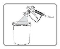
Paint should work itself from Suction Tube to Sprayer to Priming Tube until paint discharges from Return Tube. Point gun into waste bucket and pull trigger.
