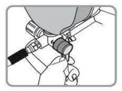
2. Switch Prime/Spray switch to Prime mode.
