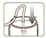
3. Submerge Suction Tube in water or flushing solvent.
