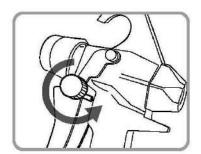
7. Release Trigger and engage Trigger Lock.
