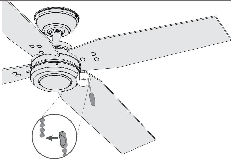
Installing the pull chain pendant - Attach the pull chain pendant to the short chain coming from the switch housing.
