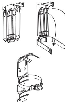
If your extinguisher has a hose and was shipped with a hose strap: Slide the hose strap over the bottom of the cylinder, and secure the nozzle end of the hose into the hose strap before placing your extinguisher in service.
