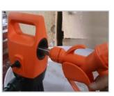
2. Place the Nozzle into the receiving container to transfer the liquid.
