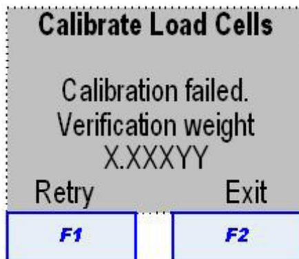
NOTE If the check repeatedly fails, check that the weights are placed on the scale properly.
