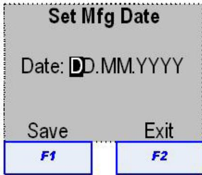
3. Enter the manufacturing date using the keypad and press Save (F1).
