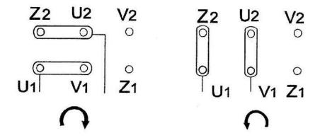
Note: The point direction is indicated to see rotating direction from the shaft extension end.
