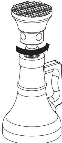
5. Rotate steel handle bar counter-clockwise to raise the lifting support until the desired height is reached.
