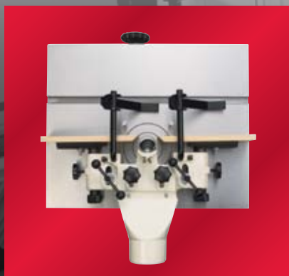
Top view of hold-downs, fence assembly and dust port features
