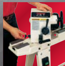
Headstock pivots 90° and locks to facilitate outboard turning
