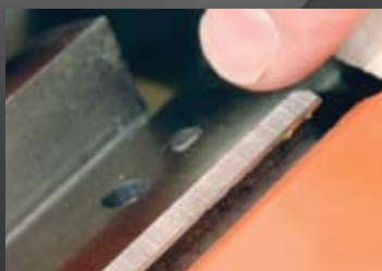
Locating pins to precisely align knives
