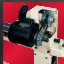
Reeves drive pulley system allows quick variable speed changes from 550 to 3,000 RPM
